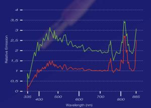
The spectral profile of xenon (and for rare gases in general) is composed of continuum of radiation - visible part from 350 nm up to 750 nm - and line radiation (atomic radiative transitions between energy levels) - IR part from 750 nm. (see figure beside) Evolution of the radiation for 2 different current densities : 3200 A/cm<sup>2</sup> and 5400 A/cm<sup>2</sup>.
