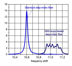
The Greitlex company has developed a method for modifying the acoustic properties of fibers. This method can significantly increase the SBS threshold (guaranteed -2 times, but typical improvement is more than 3 times) compared to a conventional fiber with the same core diameter and numerical aperture. The main advantage of our technique is that SBS-suppressed fibers are fully compatible with standard step-index fibers.
