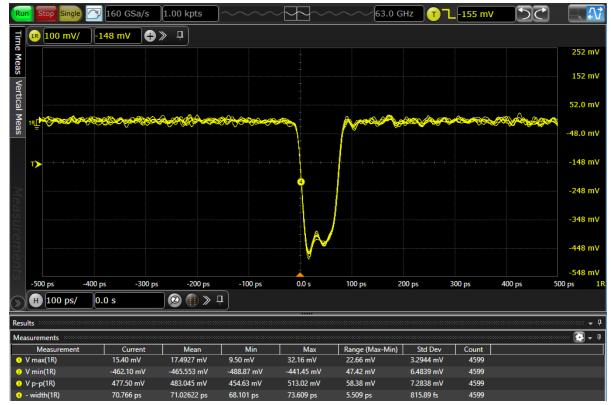
Longer pulses have a "flat top": 71 ps pulse width, amplitude  $> 400 \,\mathrm{mV}$ .
