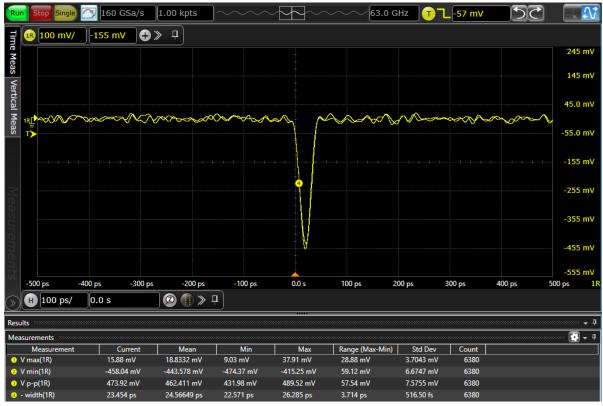
The image above shows a negative pulse width of 24.5 ps and an amplitude close to 400 mV.
