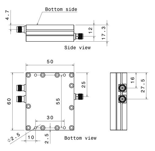
All dimensions in mm. The drawing shows the single-ended input variant (SMA plug). The differential input variant has a non-protruding SATA connector at the place where the SMA input connector is shown.
