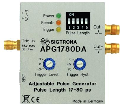
Top view of the frontpanel elements. The differential input version looks identical except it lacks the trigger level adjustment. The outputs are 2.4 mm coaxial connectors. The device can be USB powered; the power connector on the left top is optional.
