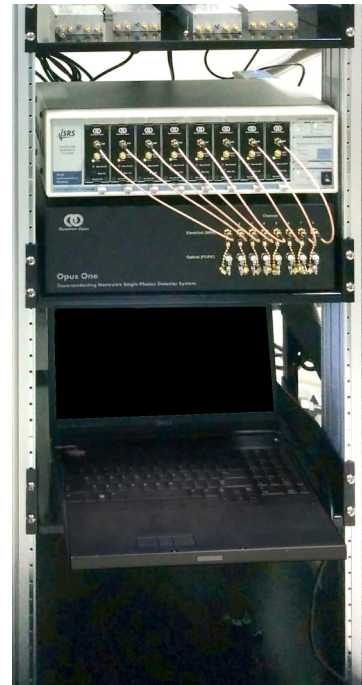
Cryostat and electronics easily rack mountable.
